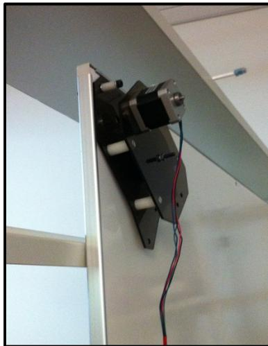
**Figure 1: First prototype of motor mounts laser cut from smoked acrylic**
